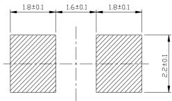
Note : Tolerances dimension  $\pm 0.1$  unless otherwise noted Angle  $\pm 5^{\circ}$  Unit : mm
