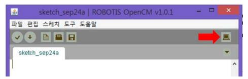
The serial monitor window can be activated by clicking on the laptop icon located on the upper right side.
