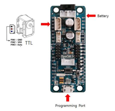
The OpenCM9.04 communicates with Dynamixel serially via Serial1 (USART1).
