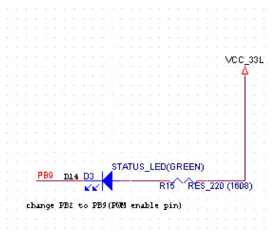
When D14(PB9) is high the LED is off; when low the LED is on.
