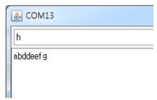
Any keyboard input is returned exactly as output.
