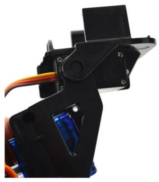
7. Fix the side servo blade to make it connect to the second servo. (The servo blade needs to be cut a little bit).
