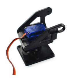
5. Fix the second servo onto the camera plate.
