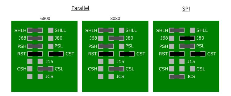
The components marked in black (marked with X in the table) are Don't Care components. This means that it does not matter, where these components are set.
