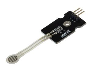
This pressure sensor works by means of analog resistance detection, when external pressure is applied to the sensor, the resistance and thus the voltage of the analog signal changes. The sensor is highly sensitive, and the sensor strip is waterproof and flexible.
