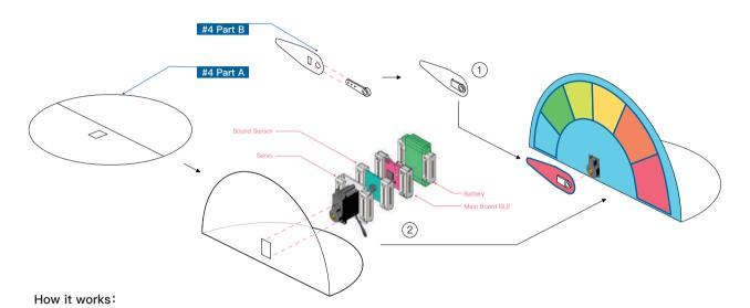
Main Board BLE: Receives sensor data from the Sound Sensor (range from 0 to 1023), then maps it to the angular position of Servo (range from 0 to 180).
