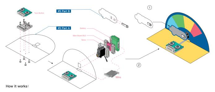
Main Board BLE: Receives button events from Twin Button, then sends the control signals to Servo.
