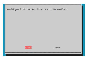
Finish the activation of the SPI interface "OK" and close the configuration with "Finish".
