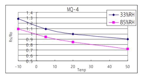
Correlation between sensor resistance and the ambient temperature and air humidity
