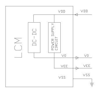
$VDD-V0(V_{LCD})$ :LCD Driving voltage
