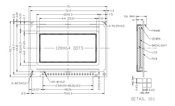
UNLISTED TOLERANDE IS ±0.5 THE MATERIAL IS LEAD-FREE.
