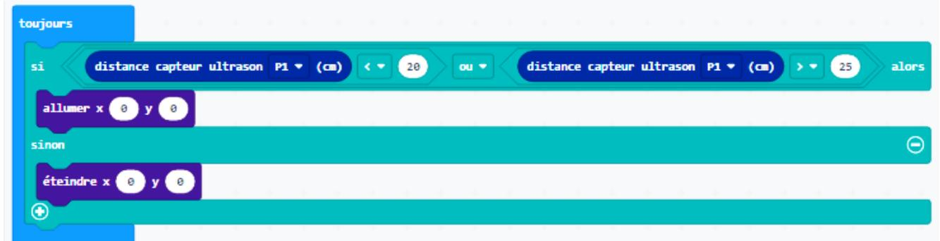
The code for Niv2 is a 'toujours' loop containing an 'si' block with the condition 'distance capteur ultrason P1 (cm) < 20 ou distance capteur ultrason P1 (cm) > 25'. The 'alors' branch contains an 'allumer x 0 y 0' block, and the 'sinon' branch contains an 'éteindre x 0 y 0' block.
