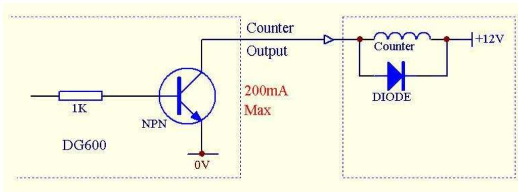
Counter output consists of a open-collector NPN transistor , on acceptance of enough coins ( no less than machine charge amount), NPN transistor is turned on to short circuit for a period of 25ms/45ms/65ms/100ms (+/-20%).here output voltage should be less than 0.7V and max 200mA is available for electric current.
