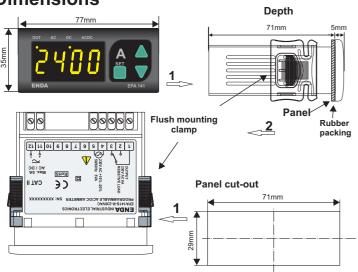
For removing mounting clamps:
