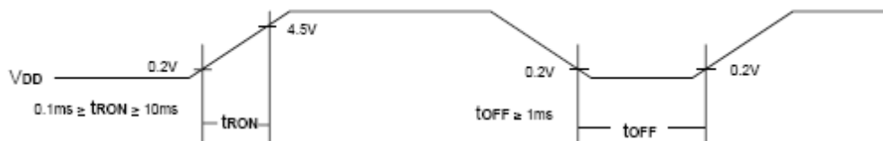
Figure 3. tOFF stipulates the time of power OFF for instantaneous Power supply to or when power supply repeats ON and OFF
