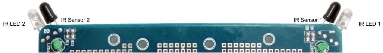
These sensors are numbered 1 to 4 for easy identification. Each sensor consists of an IR LED and an IR phototransistor. Because you cannot see IR with your eyes a small green LED is connected to each IR LED so you can see when it is on.
