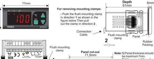
2) If there is not 60mm free space at the back side of 5m the device.it would be difficult to remove it from 29, the panel.
