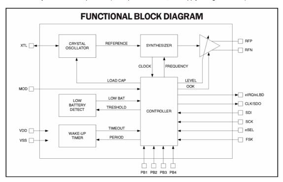
For low-power applications, the device supports automatic activation from sleep mode. Active mode can be initiated by several wake-up events (on-chip timer timeout, low supply voltage detection).
