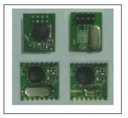
RF design, and its rapid settling time allows for fast frequency hopping, bypassing multipath fading and interference to achieve robust wireless links. In addition, highly stable and accurate FSK modulation is accomplished by direct closed-loop modulation with bit rates up to 115.2 kbps. The PLL's high resolution allows the use of multiple channels in any of the bands.
