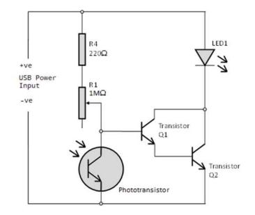
The circuit operation is very simple. When the input to the transistor Q1, which is fed from the connecting point of R1 and the Phototransistor, is greater than 1.4V, the output is turned on. Normally it requires 0.7V to turn on a transistor but this circuit uses two transistors in a Darlington Pair, meaning that it requires  $2 \times 0.7V = 1.4V$  to turn on both transistors.
