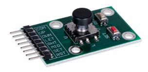
This navigation switch has 5 directions (left, right, up, down, push), as well as two additional buttons. All contacts are conveniently closed via a common ground pin.
