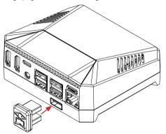
8 Connect the cables at the Back. Do not forget to **PRESS** the Power Button to **Turn ON**.
