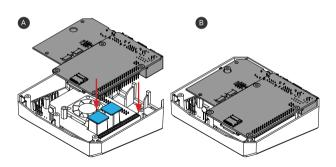
3 Use shorter **flat head screws** to fasten Raspberry Pi and HDMI Board assembly to top case.
