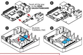
Reminder: Peel off plastic on both sides of the thermal pad
