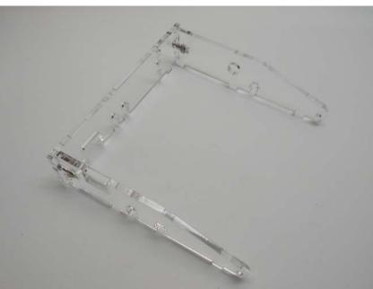
Remove the protective film from the acrylic parts. Attach the lift servo to lift servo panel (D) using two M2x10 machine screws [3] and M2 nuts [3]. Attach the servo horn to the servo shaft using the M2.5 machine screw packed together with the servo accessories.
