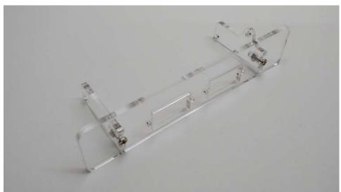
Mount both servo motors using M2x10 machine screws and M2 nuts.
