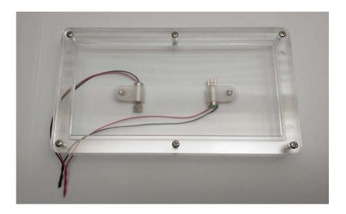
Now tighten the screws until the vibration motors are firmly in place and the clips cannot rotate easily anymore. You can try different alignments of the vibration motors to discover how it effects the distribution of the sand while vibrating.
