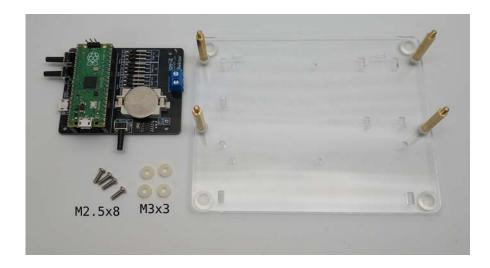
Note that the screws are tapped into the base plate, nuts aren't required.
