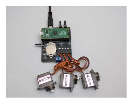
Connect the power connector to the shield PCB and the Pi Pico to your PC via a USB cable. If it asks you to install the boards drivers (usually when it's connected for the first time), do it.
