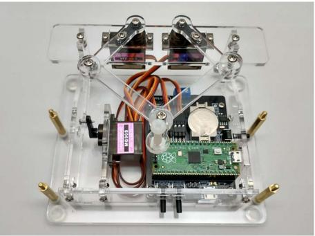
Remove the protective film of the acrylic parts of the sand box (M), (N) and (O). Screw the panels together using 6 M2.5x12 machine screws. Make sure the panels are secured firmly against each other without over tightening the screws.
