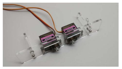
Attach the pantograph servo mechanism to the base of the clock using 2 M3x10 machine screws and 2 M3 lock nuts. Tighten the screws so the pantograph mechanism can rotate freely with as little slack as possible. Route the servo wires under the lift servo and connect them to the shield PCB. Turn the pantograph servo mechanism upright and attach it to the lift servo lever using an M3x10 machine screw and a M3 lock nut. Tighten so the mechanism can operate freely with as little slack as possible.
