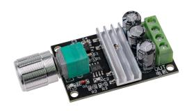
This PWM motor controller allows you to easily and smoothly regulate the rotation speed of your motor. Input and output are provided with convenient screw terminals so that the power supply and motor can be easily connected to the controller.
