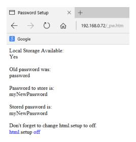
The password is now loaded on your browser. Do the same for any further browsers you want to enable. When you have done uncheck the "Enable \_pw.htm" box to prevent anyone else from loading the password. When the "Update Pending" light goes out re-boot the module again.
