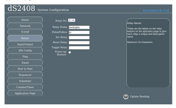
Use the Relay No. box to select the relay to configure. There are 32 relays available. Relays 1-8 are the physical relays on the module. Relays 9-32 are virtual relays, they have no physical presence but otherwise behave the same as the real ones. I/O lines may be linked to virtual relays to provide additional physical outputs, see next section for details.
