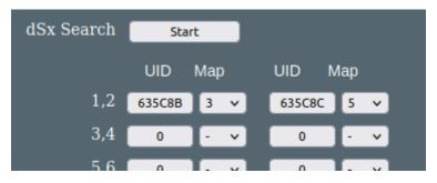
Next change the mapping as required to 29 for the first module and 31 for the other, using the drop-down selection boxes.
