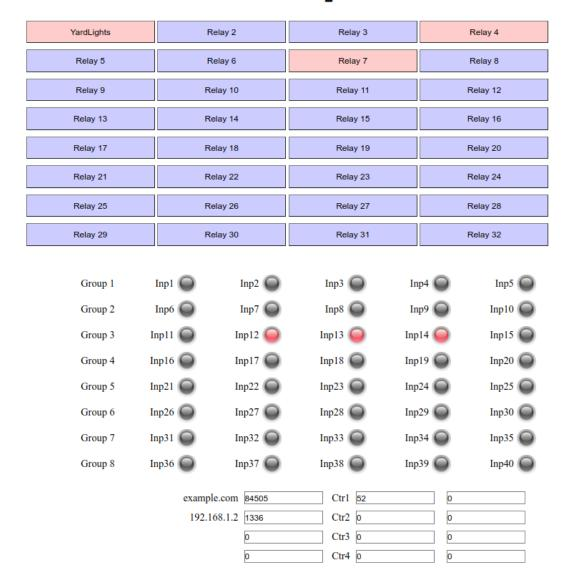
The I/O indicators show gray when the I/O is inactive. Red indicates an active input/output.
