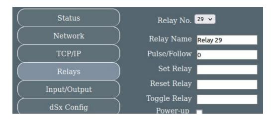
If you want, you can give the relay a more descriptive name. To use input 161 as an analogue input we use A161. If we wanted a digital input it would be D161. Enter the following into the Pulse/Follow box:
