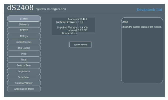
This status page shows you the system and application firmware revisions as well as the supplied voltage to the board and its internal temperature.
