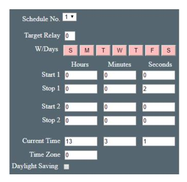
The target relay is set to zero as we don't need to use any relays for this. All week days are set so we perform the synchronization every day. Start/stop time 1 is used to activate the schedule at 1 second past midnight each day. The second start/stop time is disabled as both times are identical.
