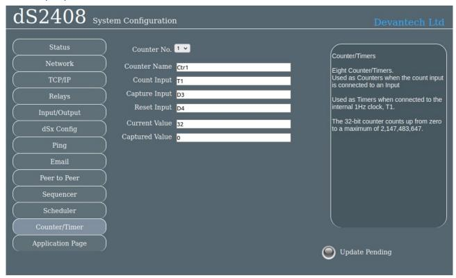
There are a total of eight counter/timers available, selected with the Counter No. box. . Each counter can count at a maximum speed of 20Hz (20 counts per second).
