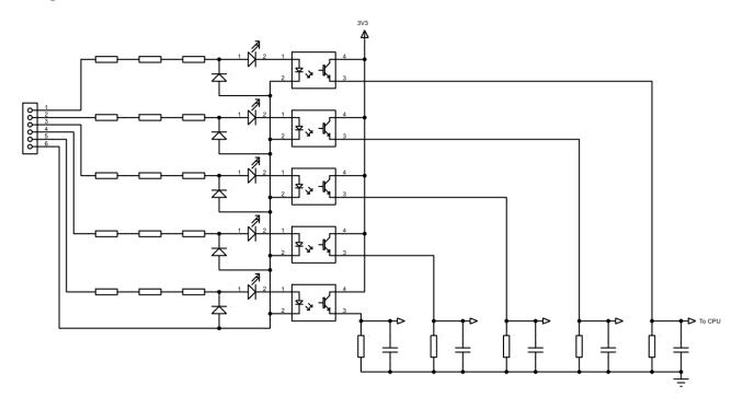
The schematic above shows a representative diagram of one group of 5 inputs, there are 8 groups for 40 inputs in total.
