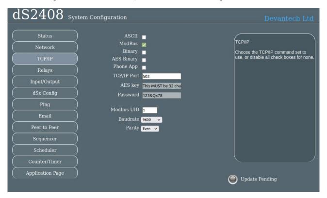
These allow you to select the UID, normally you will leave this at the default of 1. The dS2408 will respond to commands on this UID. If you send any other UID it will be treated as the address of a Modbus module connected to the RS485 port. Commands to other UID's will be converted to Modbus RTU format and sent out on the RS485 port. Any responses will be converted back to Modbus/TCP format and returned to you.
