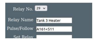
Now the relay will turn on when the input is less that 511.
