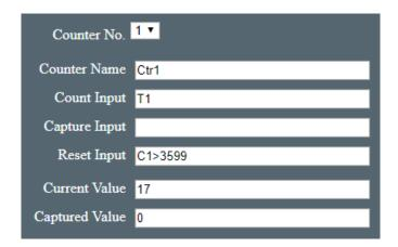
Using T1 for the count input will make the counter increment once per second. There are 3600 seconds in 1 hour so we reset the counter when its greater than 3599 with C1>3599. The counter will count from 0-3599.
