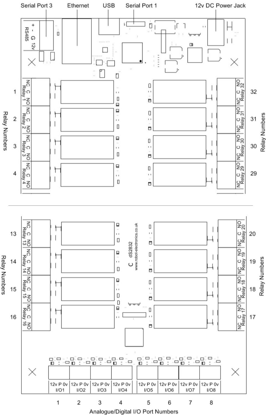
The dS2832 provides 32 volt free contact relay outputs with a current rating of up to 16Amp each, 8 flexible I/O's which can be analogue or digital and 1 serial port (3.3v level). The module is powered from a 12vdc supply which can be regulated or unregulated. The relays are SPCO (Single Pole Change Over) types. The normally open, normally closed and common pins are all available on the screw terminals.
