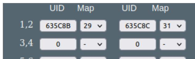
Note: the UID's are presented in ascending order, not any physical position on the RS485 bus, so you will likely need to confirm which UID belongs to which module. Clicking the UID button makes that module identify itself by flashing all its LEDs. Click again to stop.
