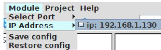
Now go to Module→ IP Address and the current IP address is displayed.
