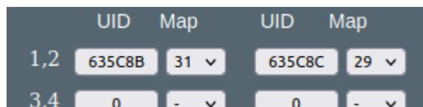
You should always design your system by mapping number, not UID. That way if you ever need to change a module you just make sure it has the same mapping as the original and your all good to go. As part of your system documentation, record the mapping number against module task so you can quickly restore the system should you need to.
