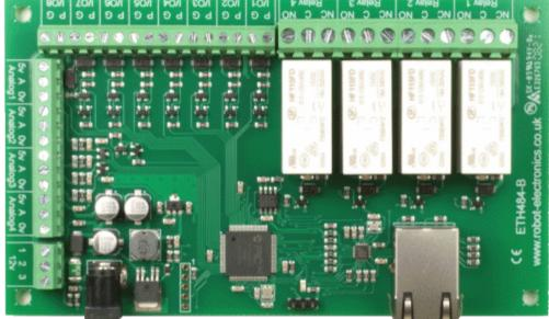
Analogue inputs 5v = 5v dc output A = Input (0-5v)0v = 0v ground
