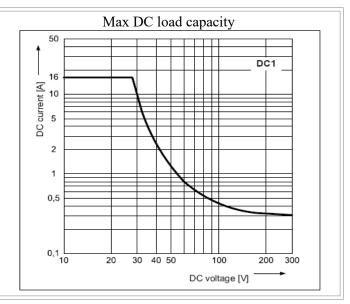
A full datasheet for the relays used on the ETH8020-B is here: HF115FD datasheet
