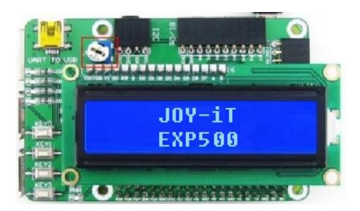
Inserting the LCD1602 into the LCD1602 interface on EXP500
