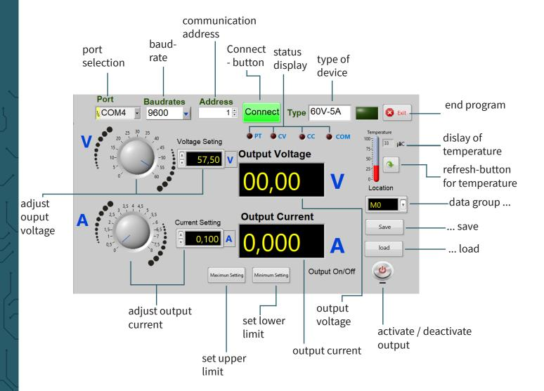
The output is deactivated if the button glows red. It will be green as soon as the output is activated.
