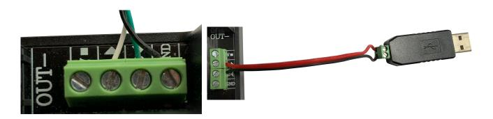
After the cable is connected with the power supply like in the picture and the chart, the device can be connected with the PC via USB. In the device-manager in point "connections (COM & LPT)", the port of the power suppy can be found. In this case, it is COM4.
