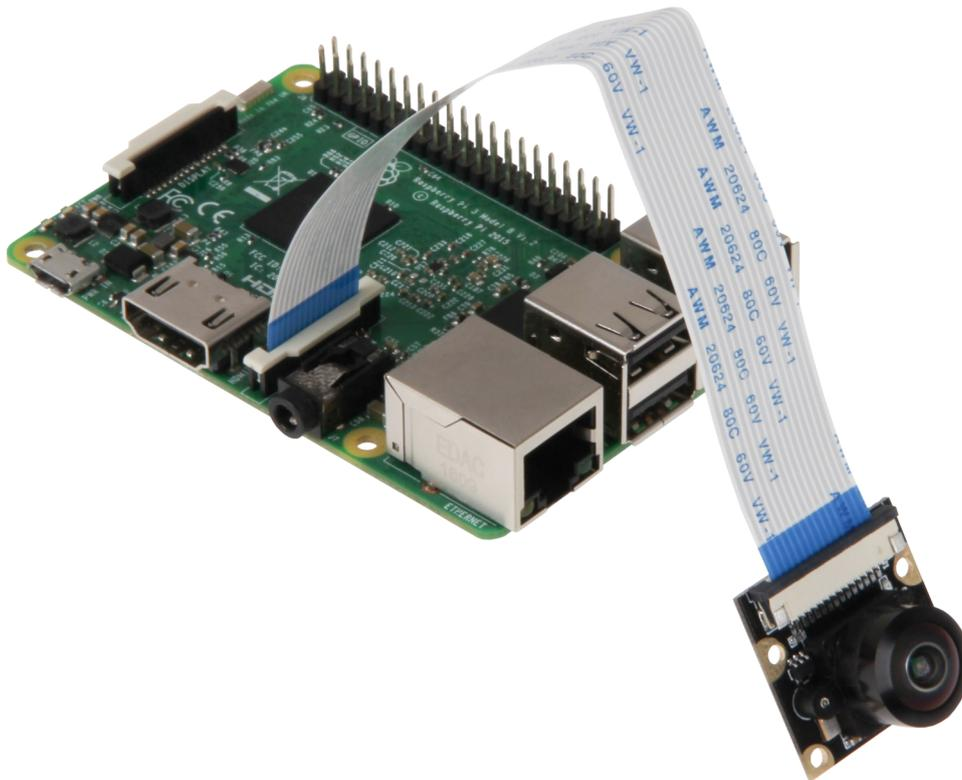
Connect the camera module, as seen in the image, with the shipped ribbon cable to the CSI interface of your Raspberry Pi.
