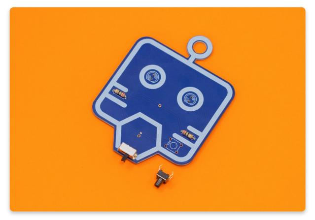
Make sure the pushbutton is placed vertically to the board before soldering.
