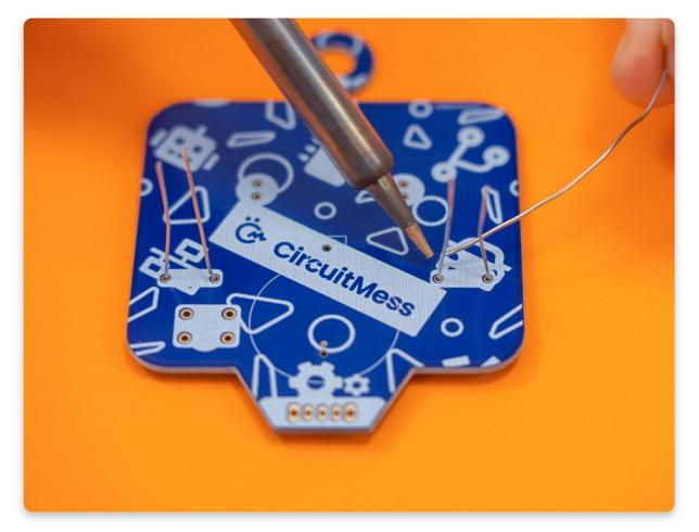
After you solder all resistors, **take one more look at the solder joints** to ensure there are no cold joints.
