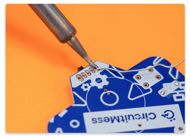
The switch's soldering joints should look like this after you have successfully soldered them:
