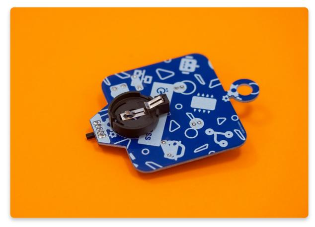
Now, turn MARV around and solder the battery holder's two pins.
