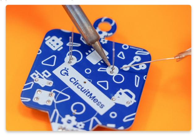
After making sure there's no bridging between the solder joints, take your pliers and cut off the rest of the LEDs' legs that you don't need.
