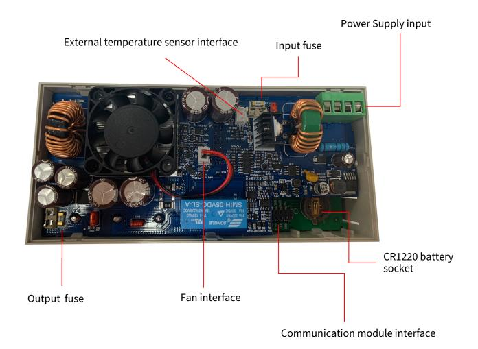
The input and output fuses are fast-blow 20 A fuses in the SMD, 6.1x2.7mm package. The sockets next to the fuses are only approved for 10 A. When replacing the fuse, you must desolder the old fuse and re-solder the new one in the same position.
