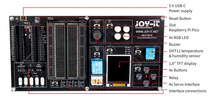
All installed components can be switched off via the respective switch if they are not needed. This way, the corresponding pins can be used for other components, if necessary.
