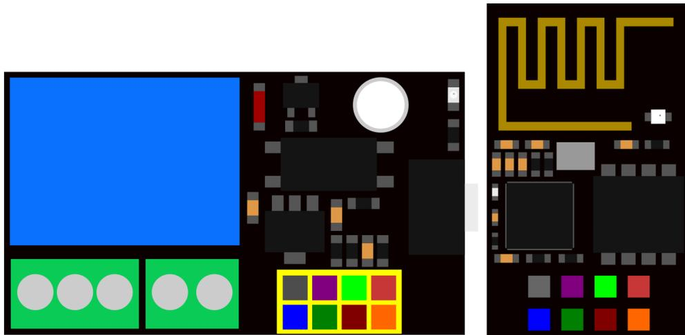
After plugging the ESP-01S into the relay module, you can now connect a supply voltage of 5 - 12 V. After that, you can go to the website by simply entering the IP address you saw in your serial output in your browser **(enter the IP address in your browser on a device that is in the same network as the ESP-01S)**.
