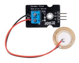
This module is equipped with a ceramic vibration sensor which emits an analog signal in case of vibration. The sensor can measure vibrations of different strengths.
