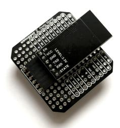
To use the WiFi GUI with your **uStepper** *S* simply load the SWiFiGUI example sketch on your **uStepper** *S* and plug in the shield!
