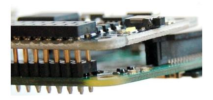
In order to make reliable connection, we suggest to use a <u>stacking pin header</u> (not included in the package).
