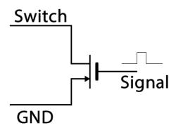
The signal should be a positive pulse, and the pulse length should be longer than 300ms. Processing a pulse will be equal to taping the switch once, so it will turn on your Raspberry Pi if your Pi is off, or turn off your Raspberry Pi if your Pi is on.
