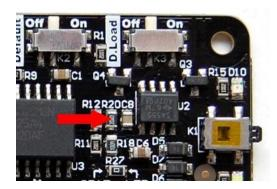
How the pulsing dummy load works? You may ask. The idea behind is quite straightforward. The SA555 chip will generate the pulsing signal, which is routed to
