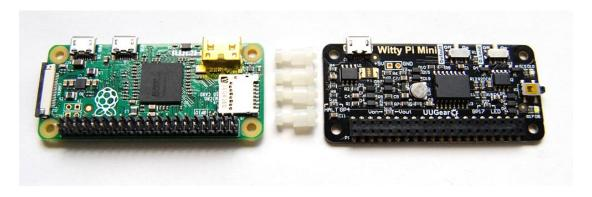
You can simply mount Witty Pi Mini on your Raspberry P Zero's 40-pin header, and it can work just like that. However, if you wish, you can use the plastic screws, spacers and nuts in the package to tightly mount Witty Pi Mini on your Raspberry Pi Zero. Please make sure NOT to put Witty Pi Mini up side down, the 40 pins should connect to the female header via the holes underneath, as shown in figure below.
