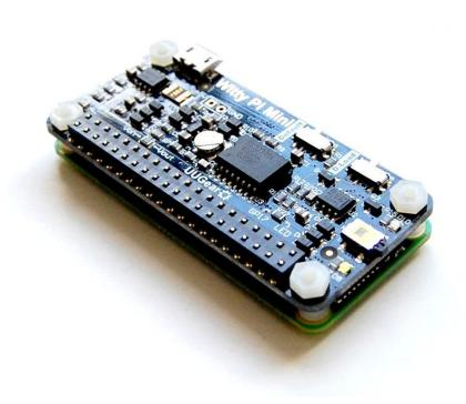
You will need to connect the power supply to the micro USB connector on Witty Pi Mini to make it work. Or you can power it via the (unpopulated) alternative power input connector.
