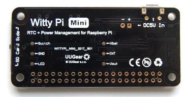
These testing pads were for product testing, but you can solder wires on them and them for extension and integration purpose.
